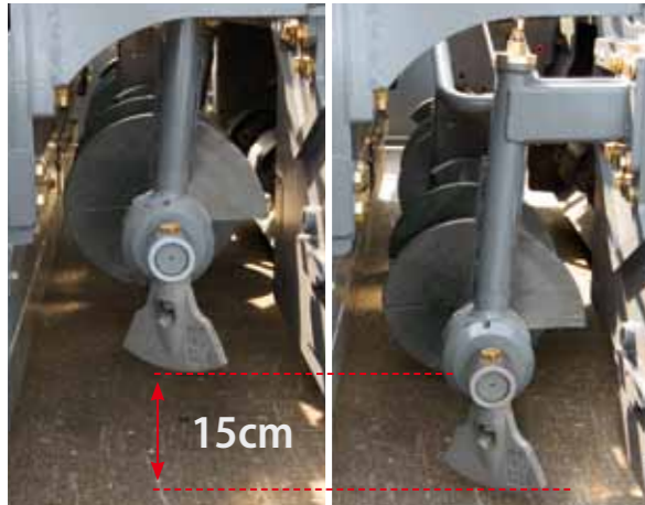
The augers of the SUPER 1900-2 are infinitely variable in height up to 15cm while paving.
