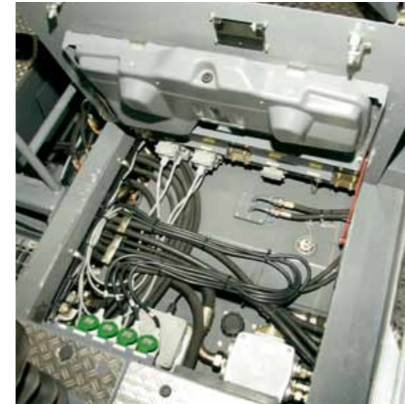
The standardized service concept conceived for the "dash 2" pavers means that servicing is quick and uncomplicated. Large hinged panels provide convenient access to all service points on the machine.
